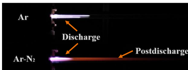
Fig. 1: Ar and Ar-N 2 plasmas generated with surfatron device.
