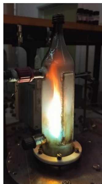
Fig. 1: Microwave plasma torch during graphene synthesis process.
