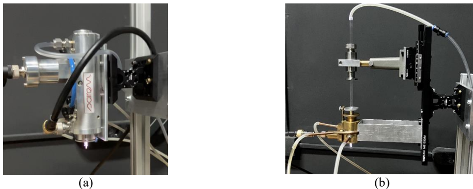
Fig. 1: (a) Sairem S-Wave Launcher; (b) Home-made S-Wave Launcher
