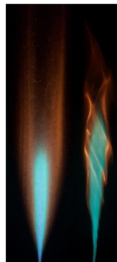
Fig. 1: Instability of torch discharge at high Q_c .
