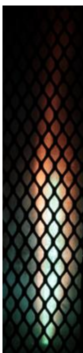
Fig. 2: TIAGO torch shielded plasma during graphene synthesis
