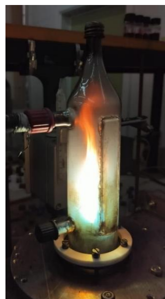
Fig. 1: Microwave plasma torch during graphene synthesis process.
